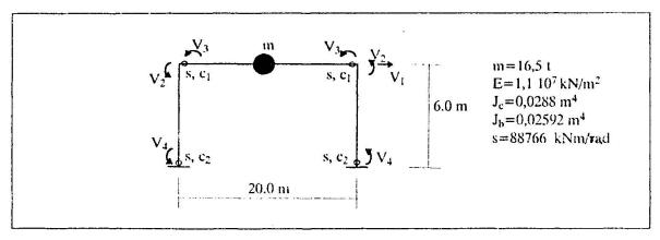
Fig. 2. Dynamic model of a one-storey laminated timber portal frame
