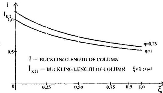
It can be noticed that for different values of fixing degree  $\eta$ , the ratio  $P_{k1} / P_{k0}$  changes already linear with changing of fixing degree  $\xi$ , that significantly simplifies procedure of designing the parameter of critical load and buckling length of columns.
