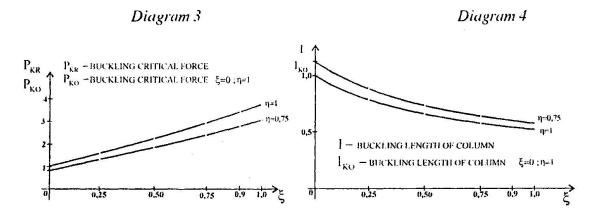
It can be noticed that for different values of fixing degree  $\eta$ , the ratio  $P_{k_1}/P_{k0}$  changes already linear with changing of fixing degree  $\xi$ , that significantly simplifies procedure of designing the parameter of critical load and buckling length of columns.
