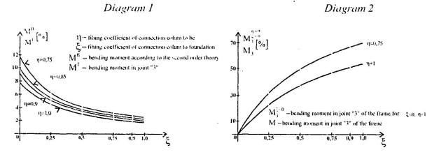
At Diagram 1, it is shown difference between bending moment in the foundation of the column (joint "3") calculated according to the first and the second order theory, for different
