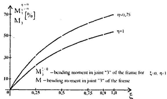
At Diagram 1, it is shown difference between bending moment in the foundation of the column (joint "3") calculated according to the first and the second order theory, for different
