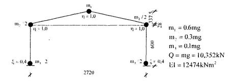
Fig. 13. Dynamically model of frame
