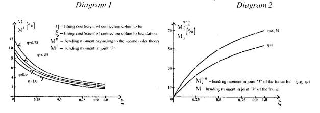
At Diagram I, it is shown difference between bending moment in the foundation of the column (joint "3") calculated according to the first and the second order theory, for different
