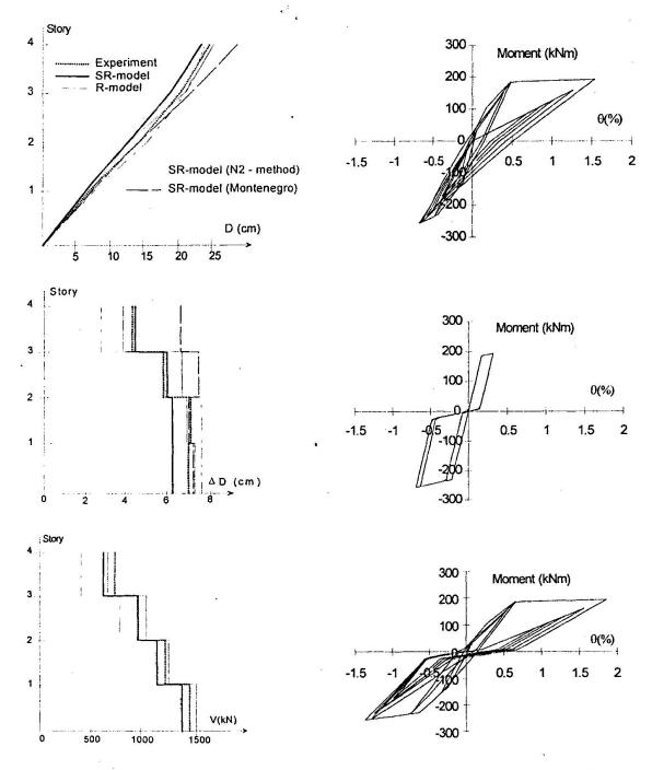
Fig. 12. Vertical distribution of maximum displacements, story drifts and shear forces
