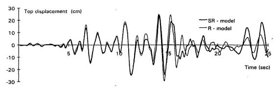
Fig. 8. Time - history of top displacement for the Montenegro based accelerogram
