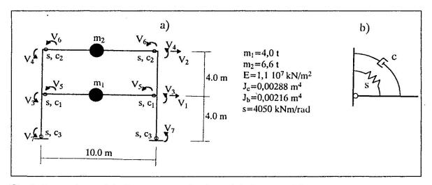
Fig. 1. Dynamic model of a two-storey laminated timber portal frame
