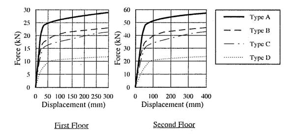
Figure 5. Load displacement relationships for the different frames
