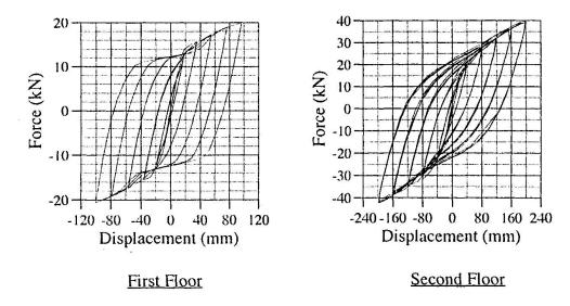
Fig. 2. Hysteretic load-displacement relationships from a cyclic test on a semi-rigid frame
