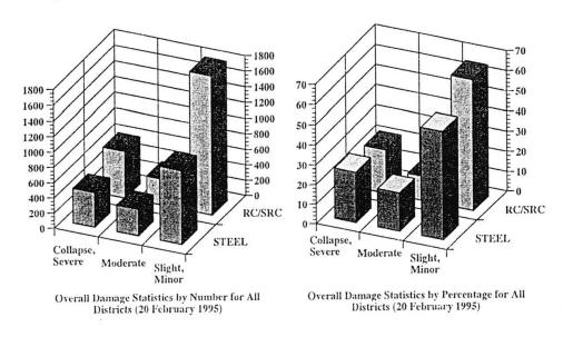
Fig.1. Damage Statistics from the Hyogo-ken Nanbu Earthquake (Elnashai et al, 1995)
