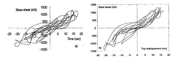
Fig. 11. Computed (a) and experimentally obtained (b) base shear - top displacement relationships
