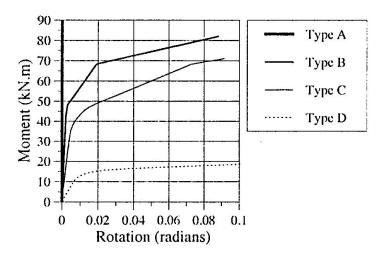
Figure 4. Moment-rotation relationships for different types of connections
