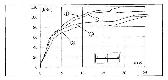
Fig. 6. M-φ curves for SCS joints
