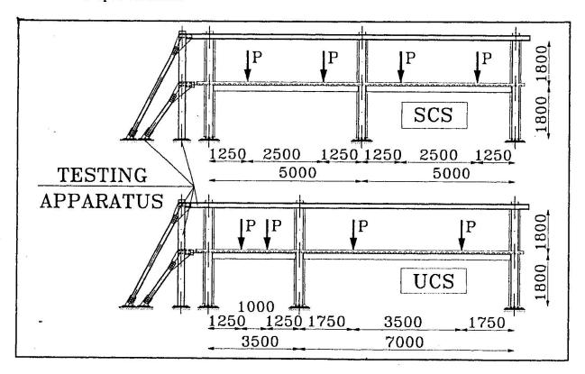
Fig. 1. Composite sub-frame specimens
