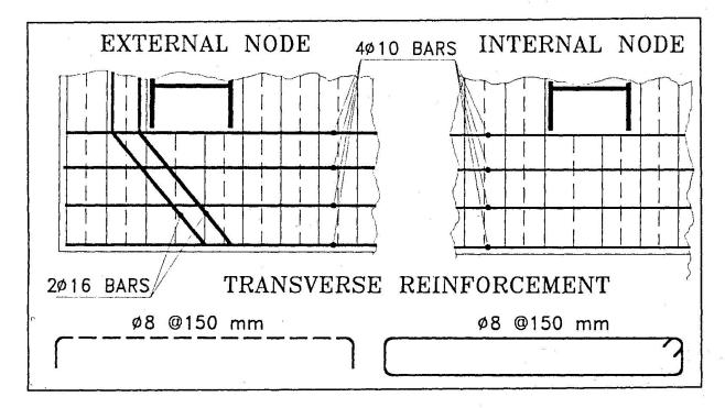
Fig. 3. Slab reinforcement
