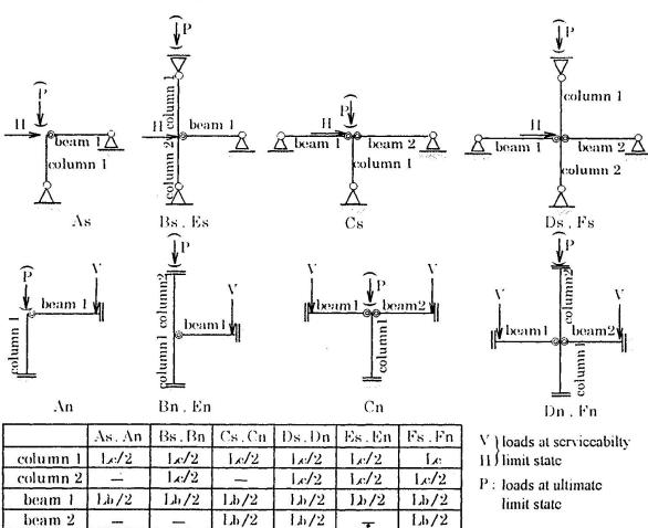
Remarks; As ~ Fs., An ~ Fn denotes the parts of multistory multibay frames shown in Fig.3
