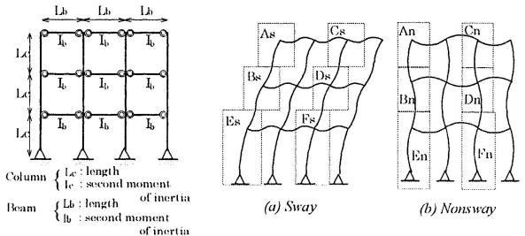
Fig. 2. Multistory and multibay frame
