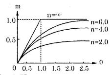
Fig. 1. Three-parameter power model
