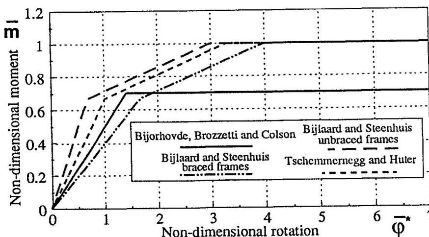
Fig. 2. Boundary curves for different classification systems.
