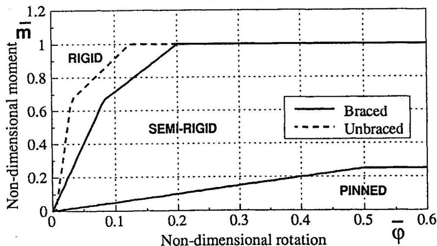
Fig. 1. Connection classification according to Eurocode 3.
