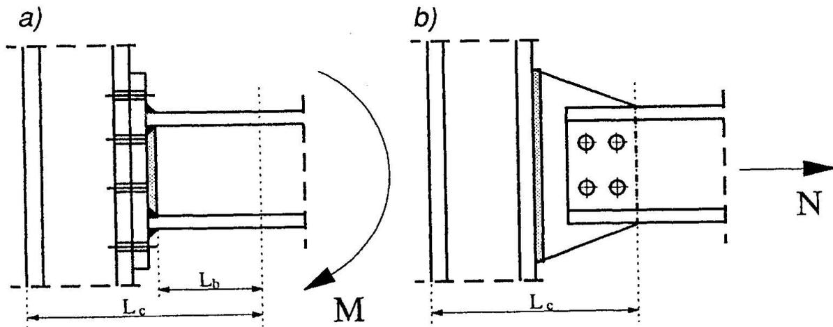
Fig. 5. Characteristic length for bending and axial joints.
