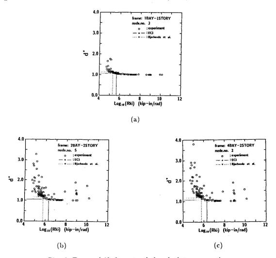
Fig. 6. Frame drift for extended end-plate connections
