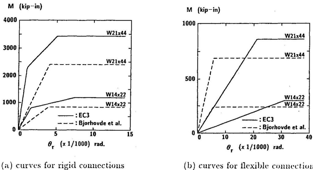
Fig. 3. Moment-rotation curves as per classification system
