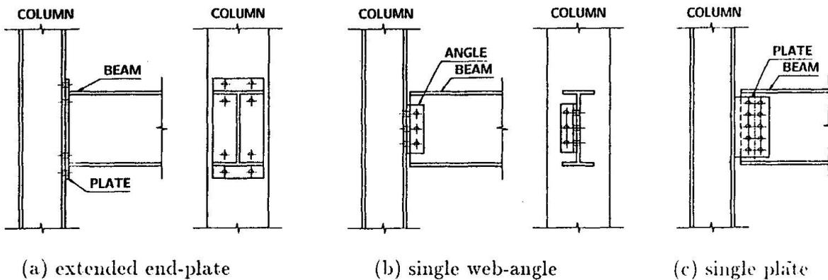
Fig. 2. Practical connections used in frame analysis
