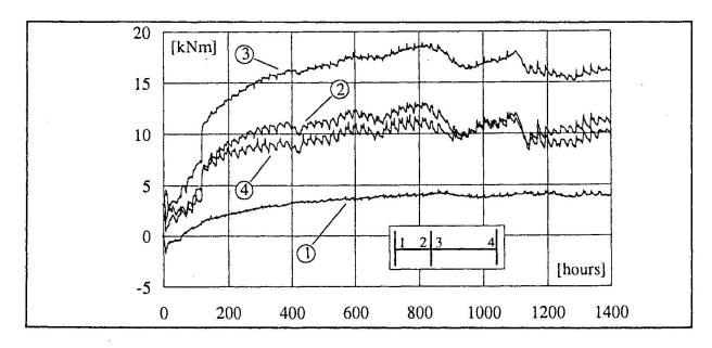
Fig. 8. Bending moments at the joints of UCS specimen before the test
