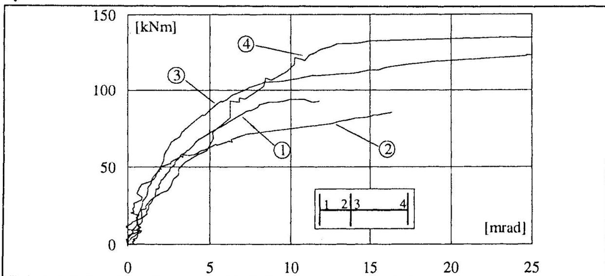
Fig. 9.  $M-\phi$  curves for UCS joints
