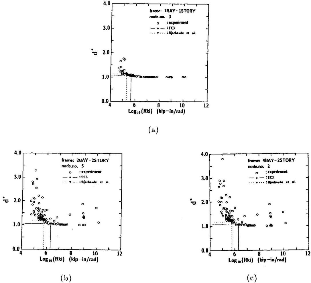
Fig. 6. Frame drift for extended end-plate connections
