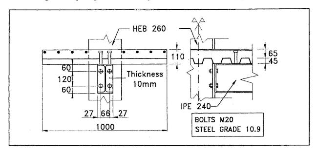
Fig. 2. Composite joint
