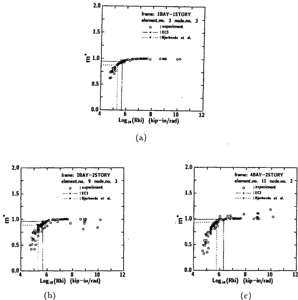
Fig. 5. Beam end moment for extended end-plate connections
