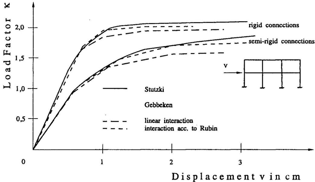
Figure 7: 2-D Frame: Load vs. deflection curves
