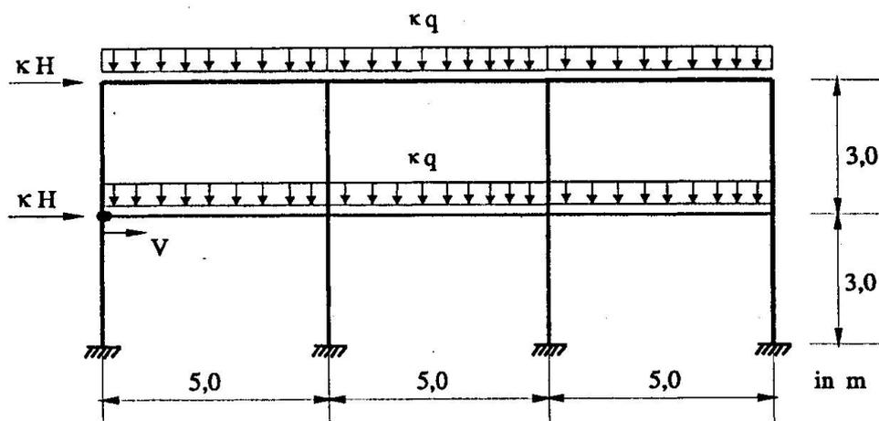
$q = 60.0 \text{ kN/m}$     Beams: HEB 300
