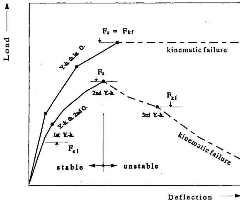
Figure 1: Comparison of load-deflection curves
