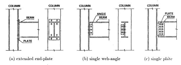
Fig. 2. Practical connections used in frame analysis
