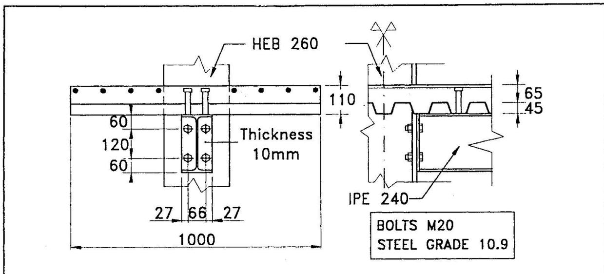
Fig. 2. Composite joint
