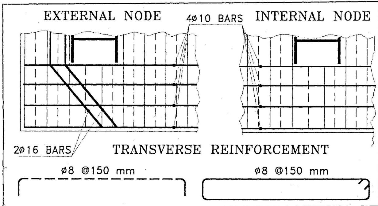
Fig. 3. Slab reinforcement
