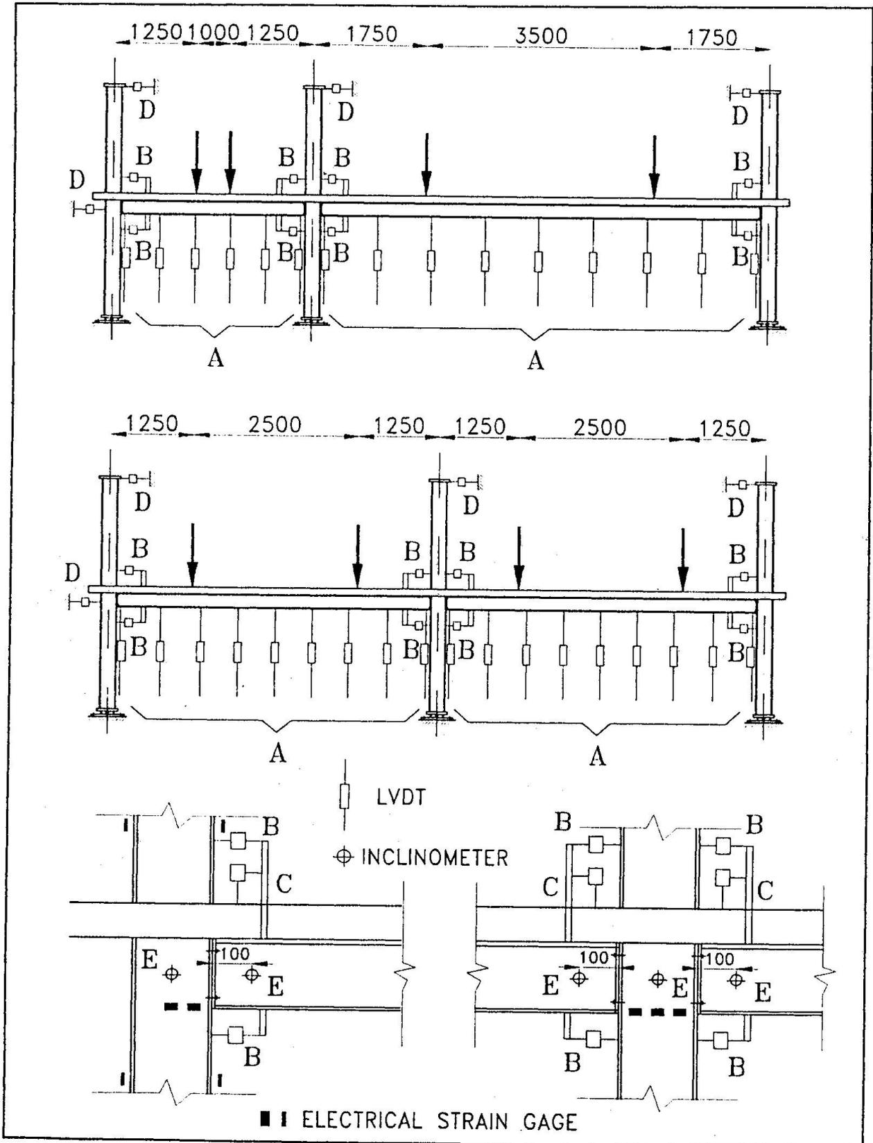
Fig. 4. Instrumentation
