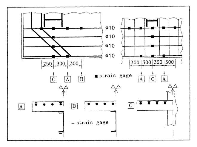
Fig. 5. Strain-gages on slab reinforcement bars.
