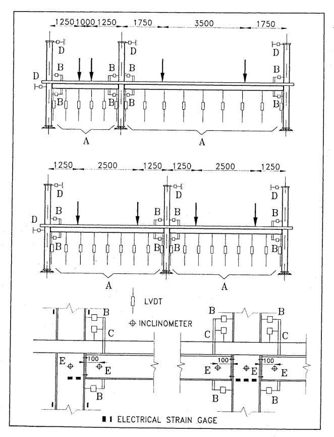
Fig. 4. Instrumentation
