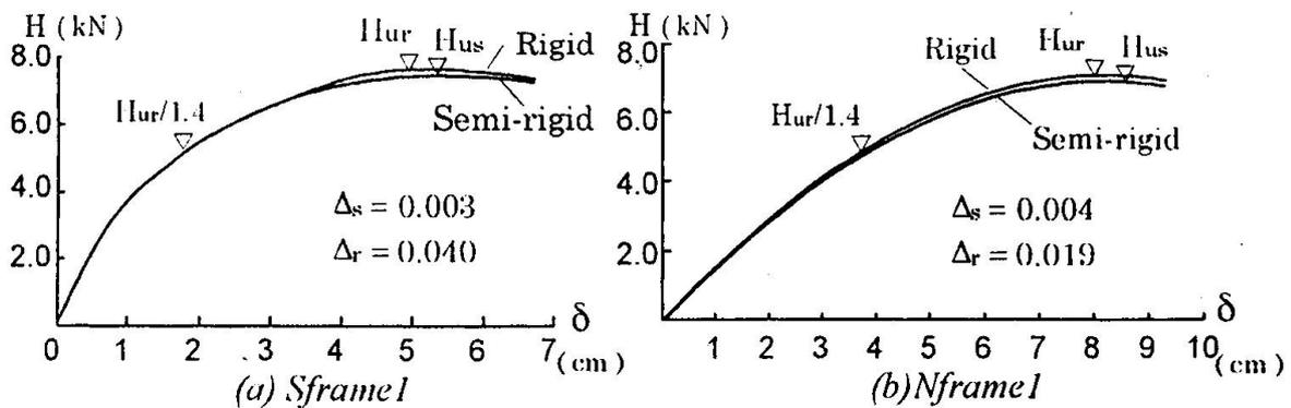
Fig. 8. Load-displacement relations
