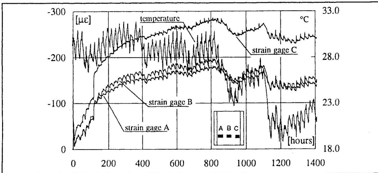
Fig. 7. Strain in the web panel of UCS specimen before the test
