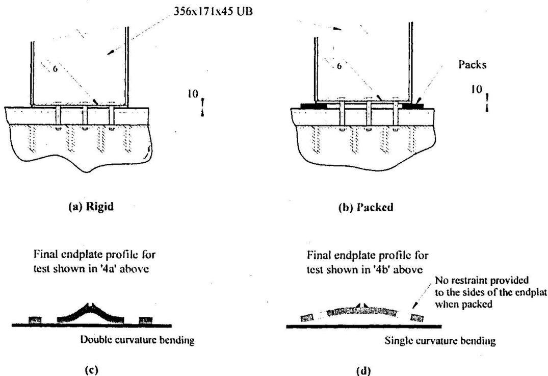
Figure 4. Details of rigid base and endplate deformations
