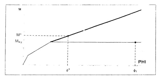
Fig. 5. Variation of the joint response with the post-limit stiffness
