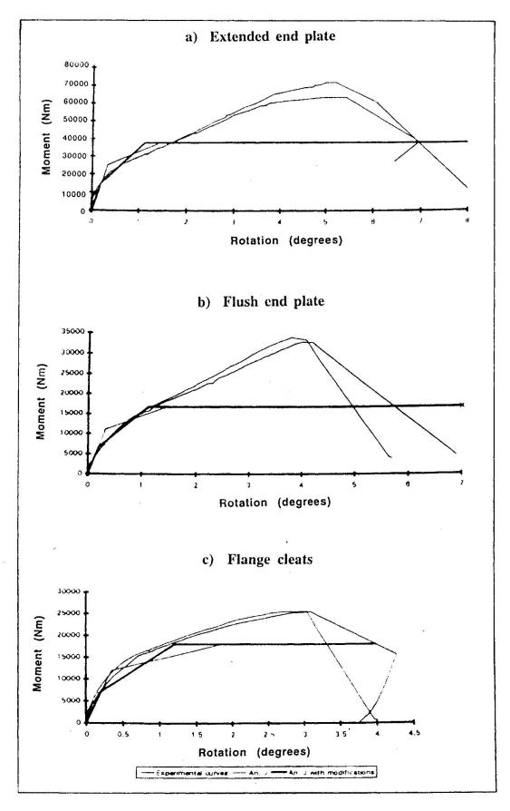
Fig. 4. Experimental curves and comparison with the curves calculated according to EC3
