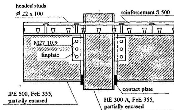
by the reinforced concrete slab stressed in tension and a contact plate between the column flange and the lower steel flange. The vertical shear force is transferred by the finplate. In practice the contact plate will be provided after concrete has hardened to establish a pinned connection during erection and to achieve significant moment-resistance and stiffness at the final composite stage. This leads to a change in the structural system during the loading history.
