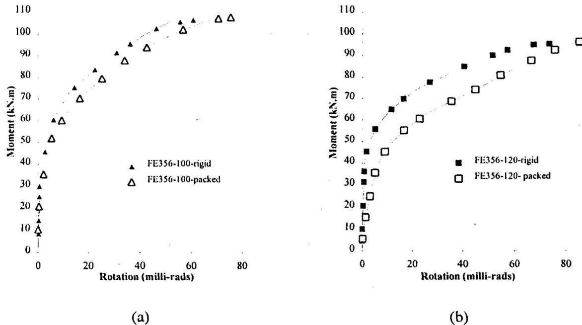
Figure 5. Comparison of Endplate moment rotation characteristics
