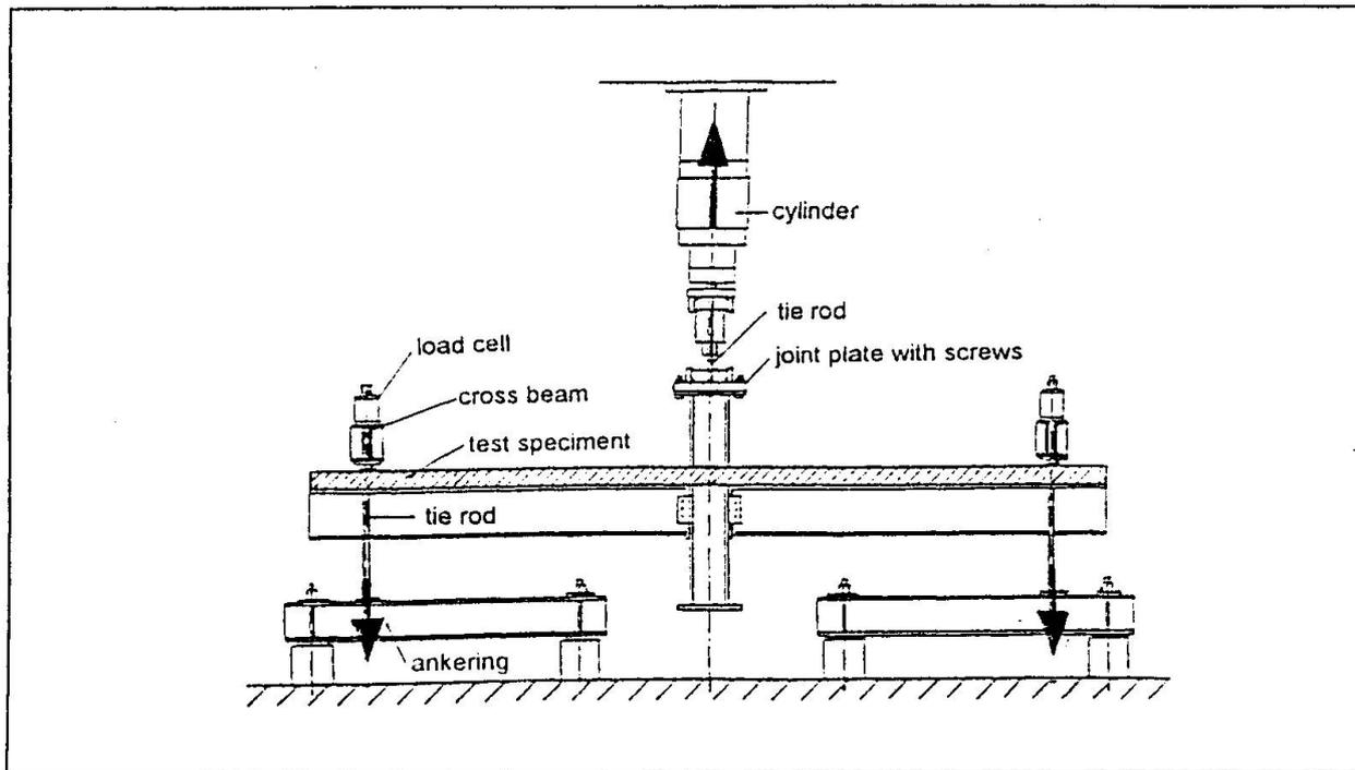
Fig. 5 Setup of the second test series
