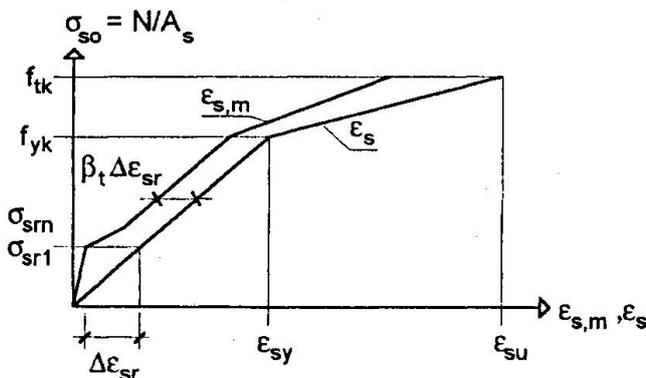
Fig. 3 Simplified stress-strain relationship of embedded reinforcing steel
