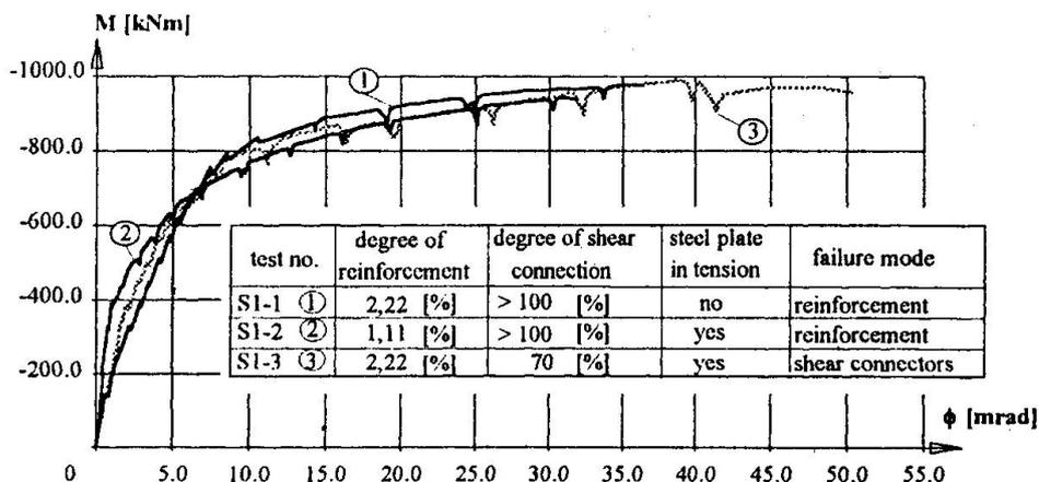
Fig. 10 Tests on composite joints with finplate connection
