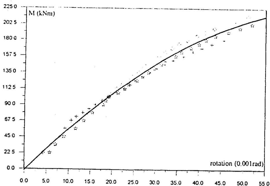
Fig.4b. (M- $\phi$ ) diagram of the weak axis connections
