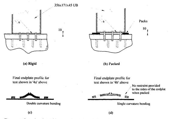
Figure 4. Details of rigid base and endplate deformations
