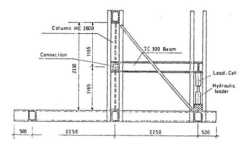
Fig.1. The test set-up
