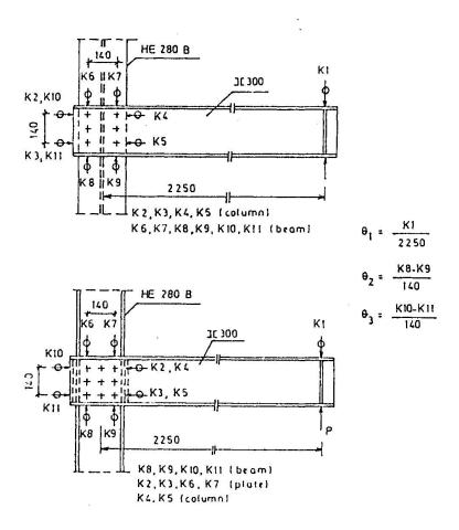
Fig. 2. Test specimens
