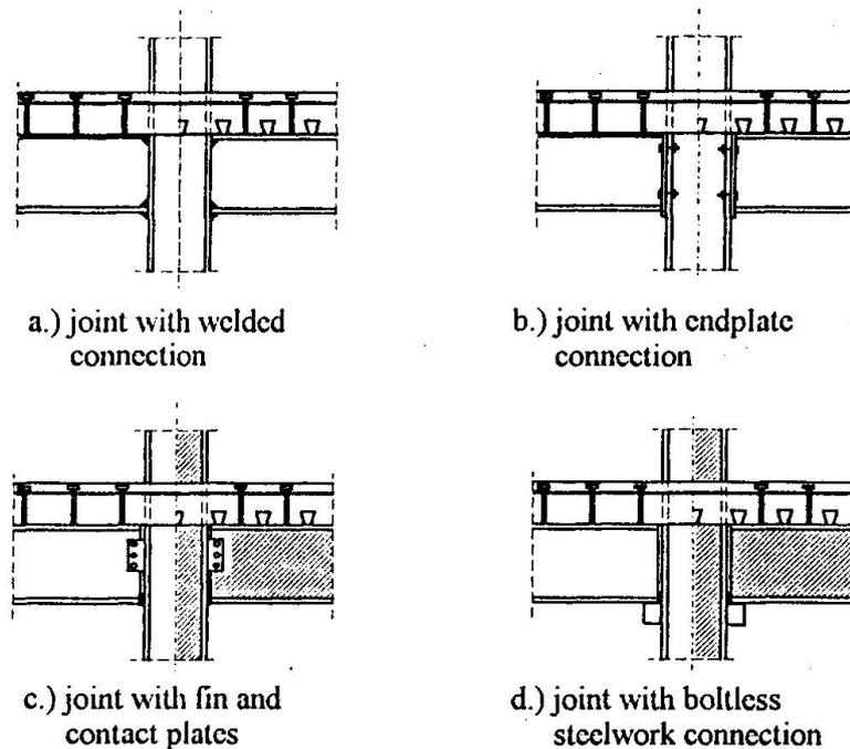
*Fig. 2 Types of moment resisting beam-to-column joints*
