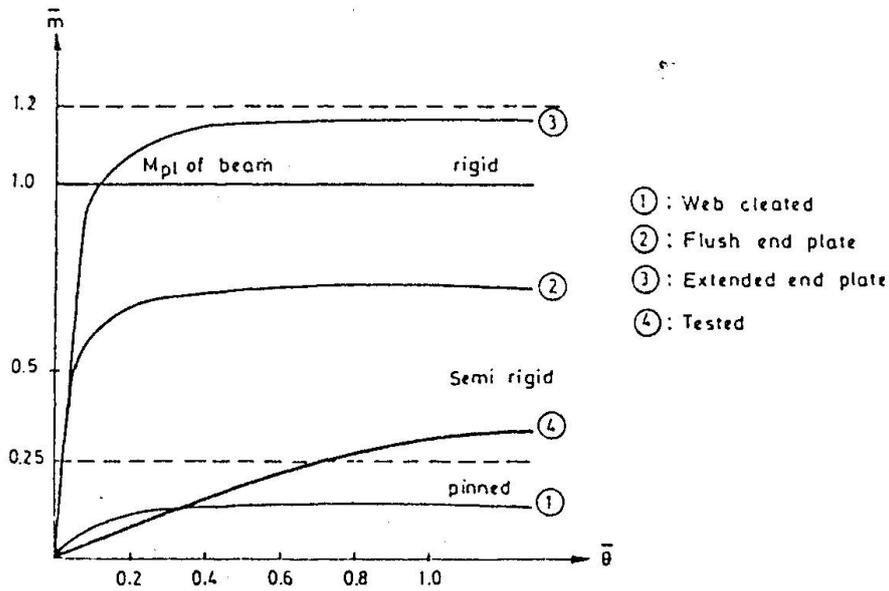
Fig. 6.  $(\bar{m}-\bar{\phi})$  diagram
