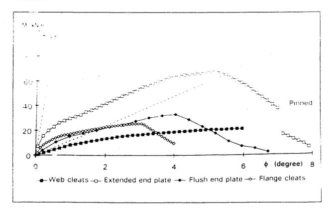
Fig. 1. Experimental curves and classification
