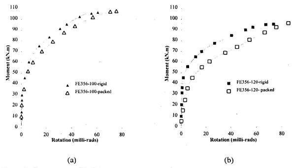
Figure 5. Comparison of Endplate moment rotation characteristics
