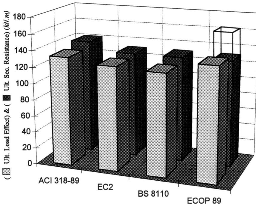
Fig. 1. Example to Show The Relation Between Ultimate Action Effect and Ultimate Section Resistance in Four Different International Codes.
