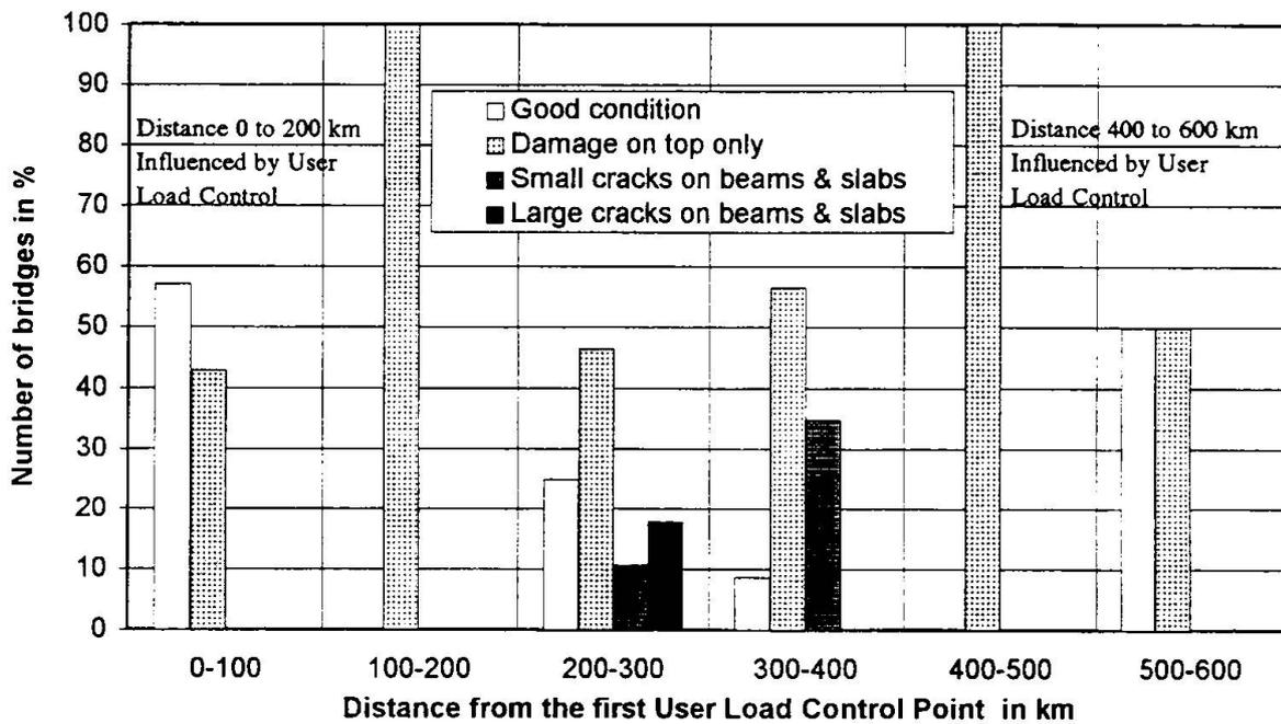
Fig. 6. Distribution of bridge damages on the 600 km road length.
