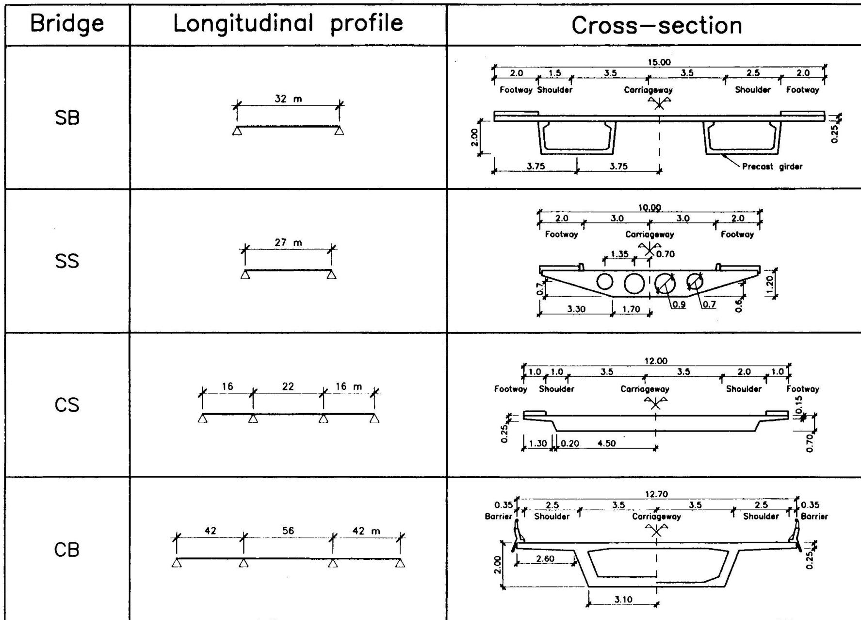
Figure 1. Layout and cross-sections of the studied bridges.
