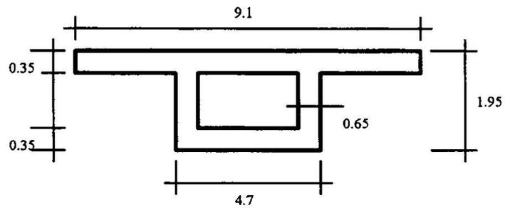
Type 1.1 (h=2.0 m), Type 1.2 (h=3.3 m), Type 1.3 (h=4.7 m)
