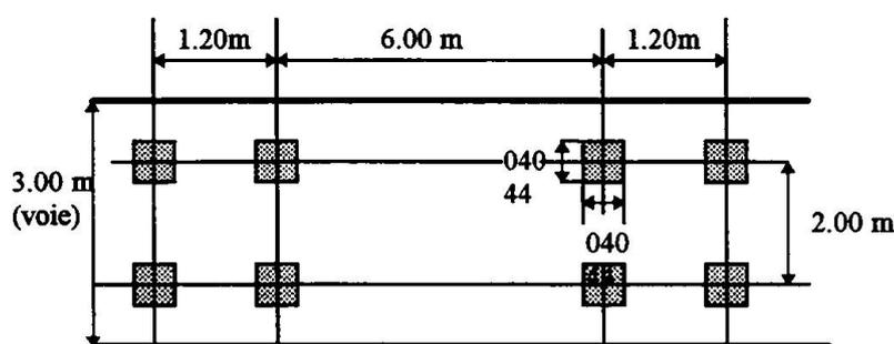
Fig. 1. Model 3 for fatigue load (Eurocode 1.3).
