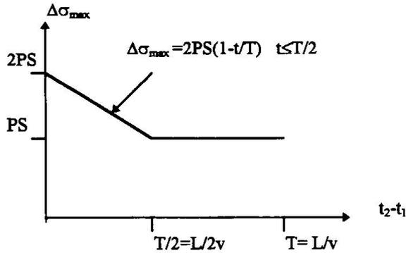
Fig. 3. Stress cycle amplitude for a passing case.
