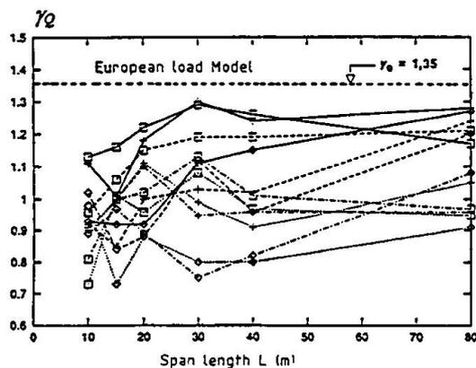
Fig. 4 :  $\gamma_Q$  values for bridge elements
