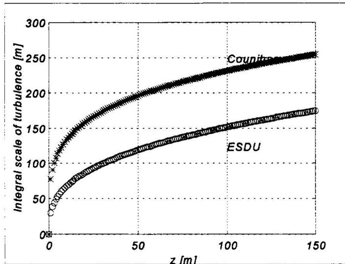
i) The length of the integral scale of turbulence from Couniham, used by Solari for EC1:
