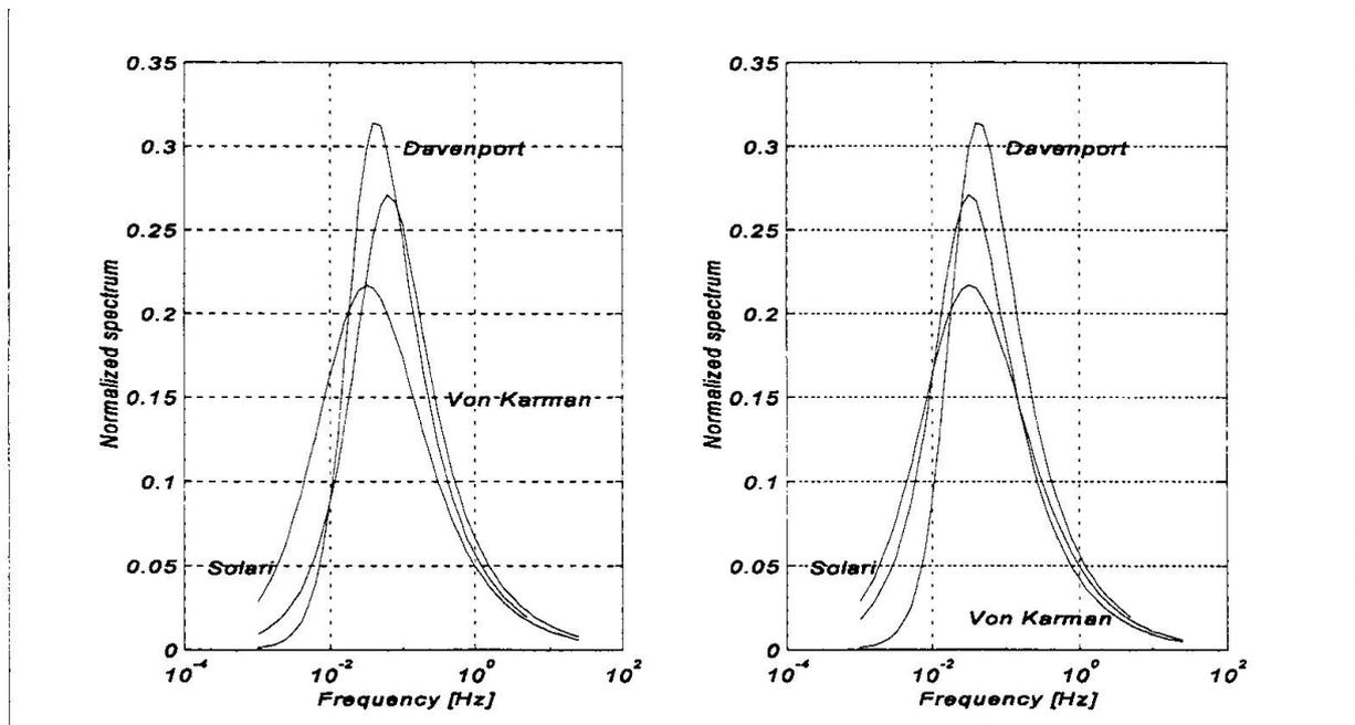
Fig. 4. Davenport, Solari and von Karman spectra at  $z=10\text{m}$ ,  $z_0=0.05\text{m}$ ,  $V_{ref}=30\text{m/s}$ , with 2 lengths of integral scale of turbulence in the von Karman spectrum; left:ESDU, right:Couniham.
