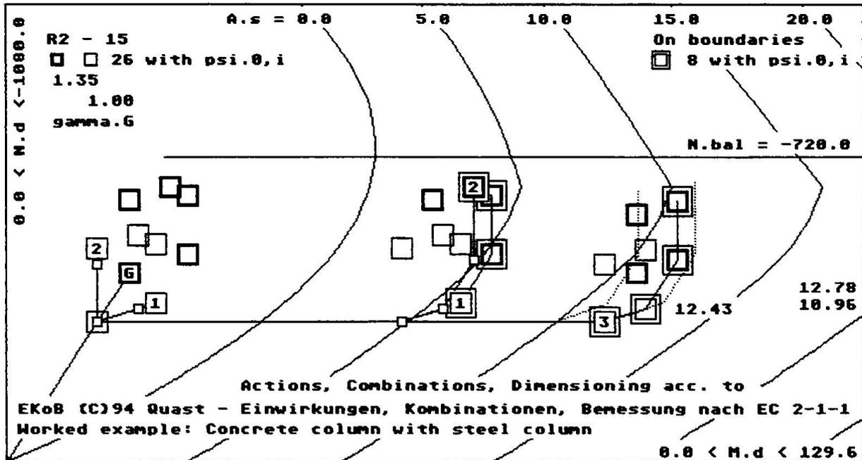
Fig. 4. Representation of the 26 combinations acc. to EC 1, eq. (9.10), within a detail of the  $N_d/M_d$ -diagram. For the vectors of the variable actions 1 to 3 the design values  $\gamma_Q \cdot Q_{k,i}$  and the design values of the combination values  $\gamma_Q \cdot \psi_{0,i} \cdot Q_{k,i}$  are marked. The 8 combinations on the boundaries, which have to be considered for dimensioning the cross section, are marked by double quadrats.
