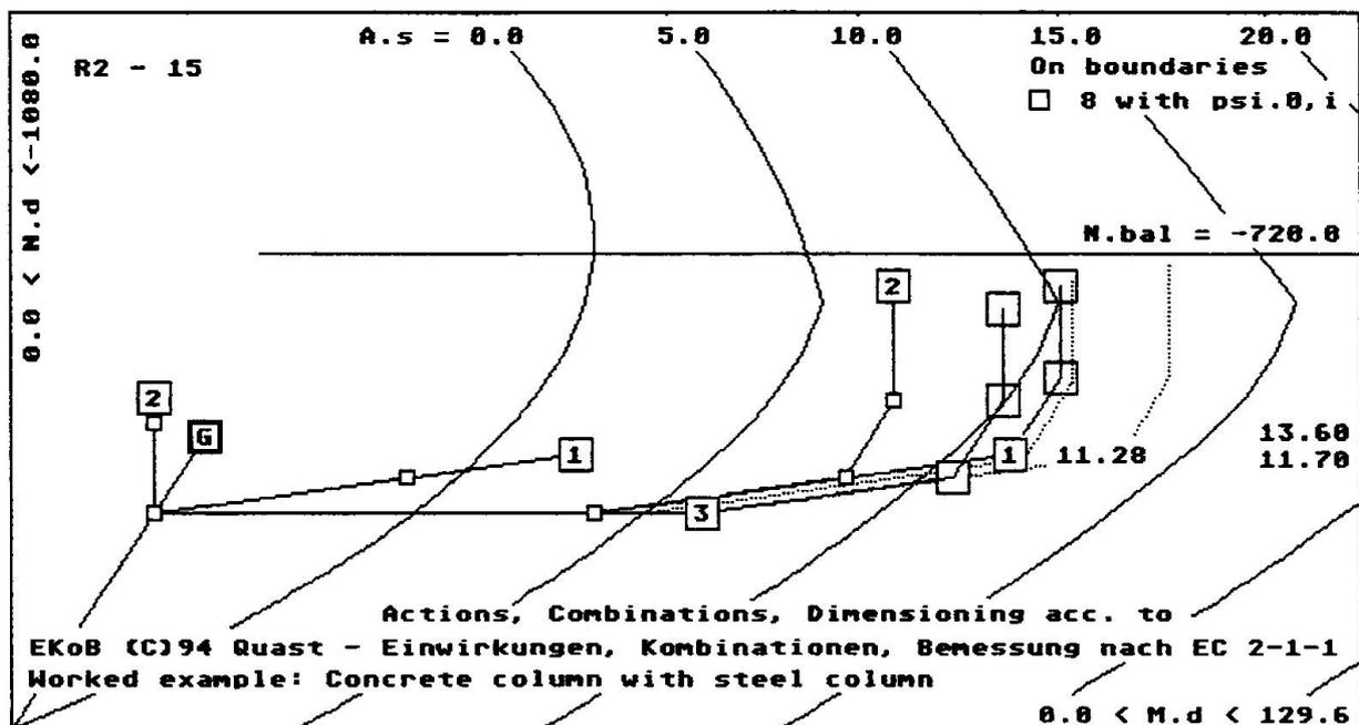
Fig. 6. Representation of the required 8 combinations on boundaries acc. to EC 1, eq. (9.10), within a detail of the  $N_d/M_d$ -diagram. Only these combinations have to be considered for dimensioning of the cross section out of a totality of 26. For the vectors of the variable actions 1 to 3 the design values  $\gamma_Q \cdot Q_{k,i}$  and the design values of the combination values  $\gamma_Q \cdot \psi_{0,i} \cdot Q_{k,i}$  are marked.
