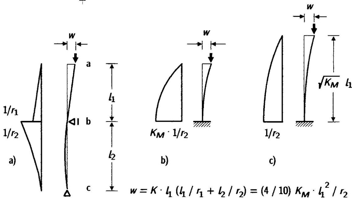
Fig. 2. Equivalent model columns for dimensioning the section b in span 2,
