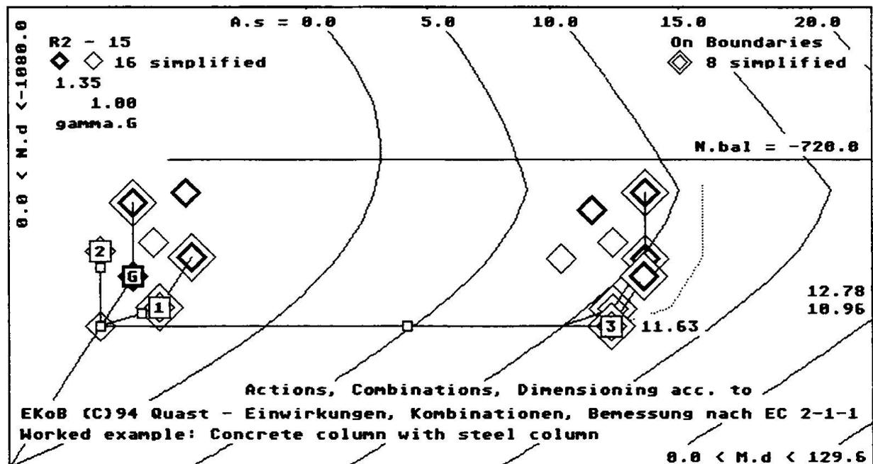
Fig. 5. Representation of the 16 simplified combinations acc. to EC 1, eq. (9.13) and (9.14), within a detail of the  $N_d/M_d$ -diagram. The 8 combinations on the boundaries, which have to be considered for dimensioning the cross section, are marked by double diamonds.
