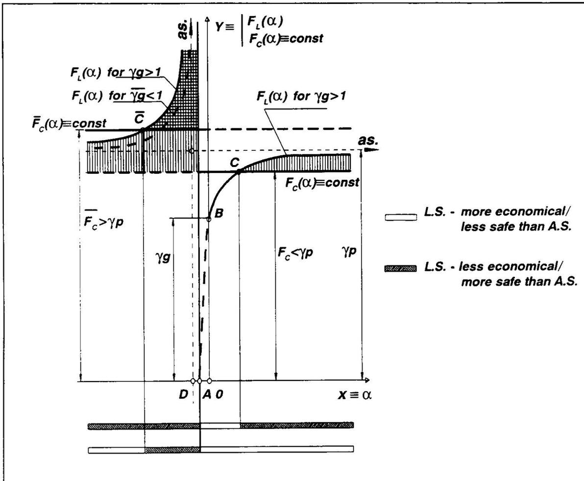
**Fig. 1** Characteristic feature of the “Safety and Economy Reciprocity” between L.S. and A.S. design by dimensioning of particular cross sections/ elements in parametric study:  $\alpha$  - Ratio of normative (without partial factors) dimensioning the temporary to the permanent forces;  $F_L$  - ratio of the acting forces (with partial factors) after L.S. to the forces after A.S.;  $F_C$  - ratio of the bearing capacities after L.S. to the capacities after A.S.;  $\gamma$  - partial factors.
