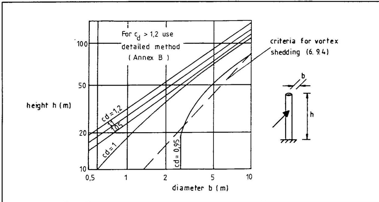
Figure 4d: Field of application for chimneys, values for reinforced concrete chimneys
