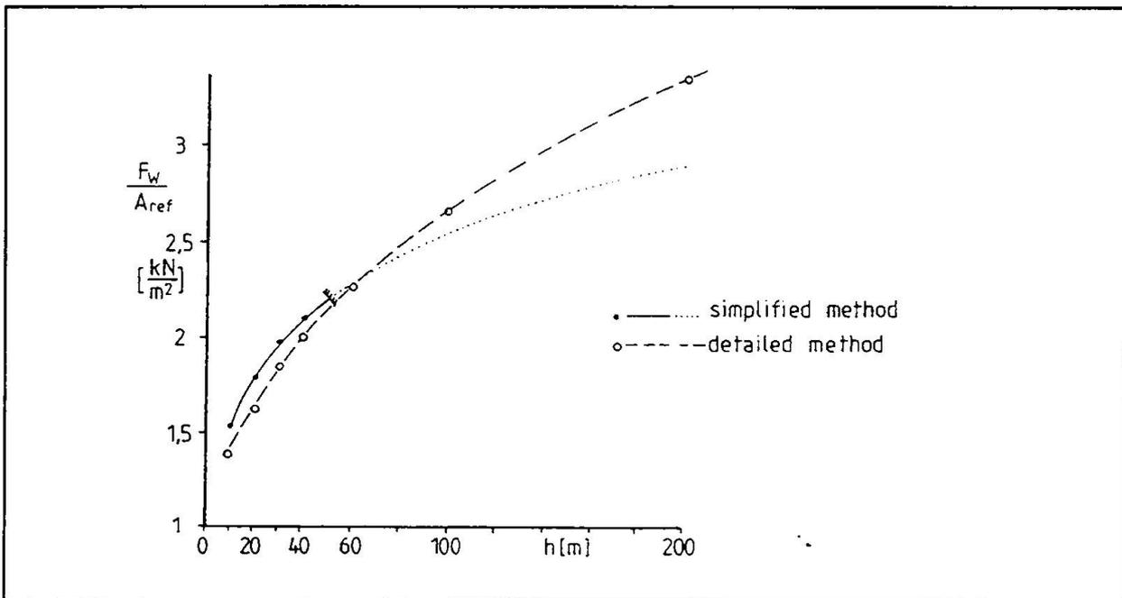
**Figure 7:** Calculated wind force per  $m^2$  for the buildings of example 5.1. Comparison of simplified method with detailed method.
