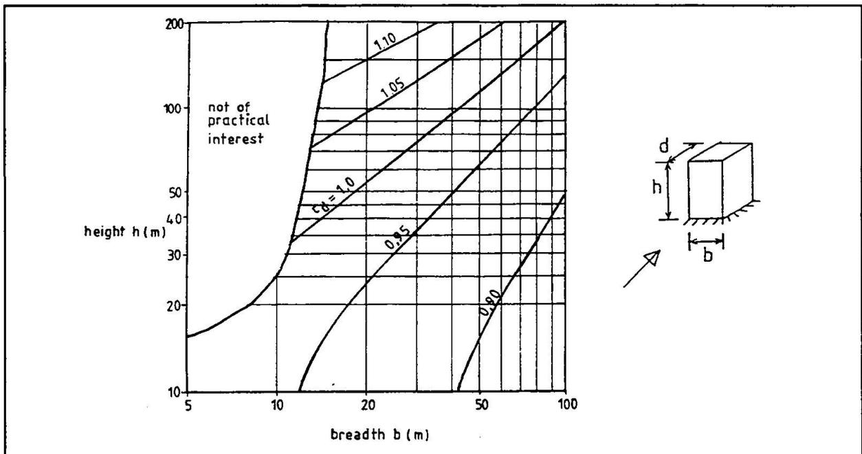
Figure 2c: Steel structure,  $\delta = 0,045 n_1 > 0,05$
