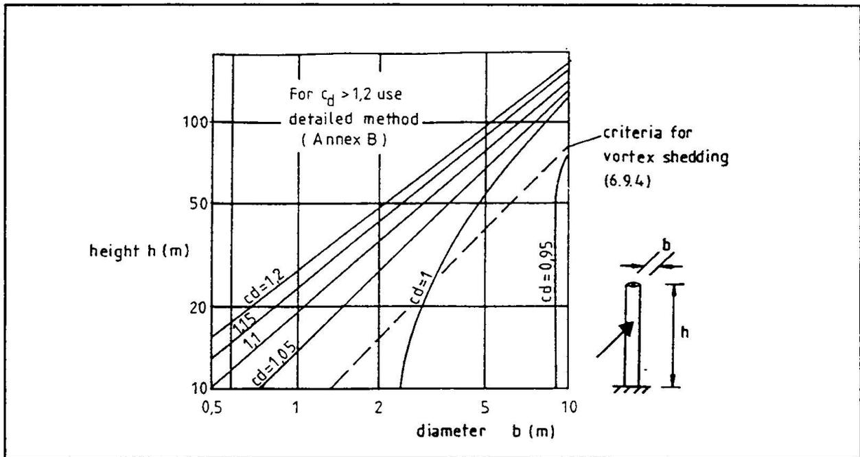
Figure 4b: Field of application for chimneys, values for lined steel chimneys
