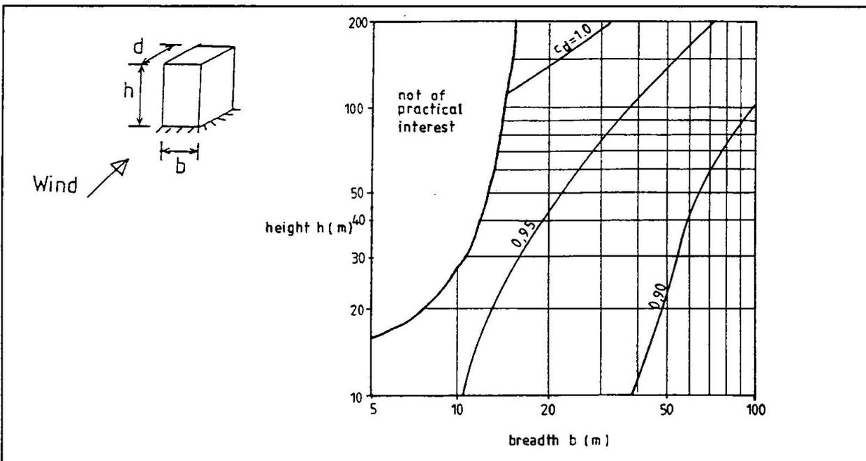
Figure 2a: Concrete structure,  $\delta = 0,045 n_1 + 0,05$
