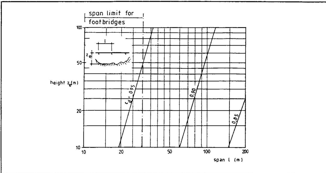
Figure 3: Dynamic factor,  $c_d$ , for roadway, railway and footbridges
