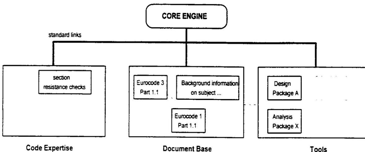
Figure 3. Integrated working environment for users of Eurocode 3
