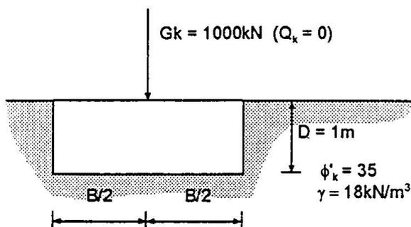
Figure 1. Centrally loaded footing.
