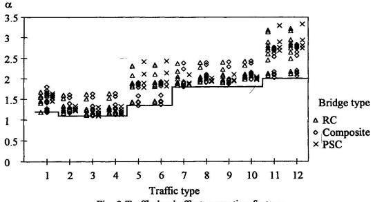
Fig. 3 Traffic load effect correction factors
