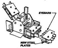
Fig. 4 Conceptual Eyebar Retrofit
