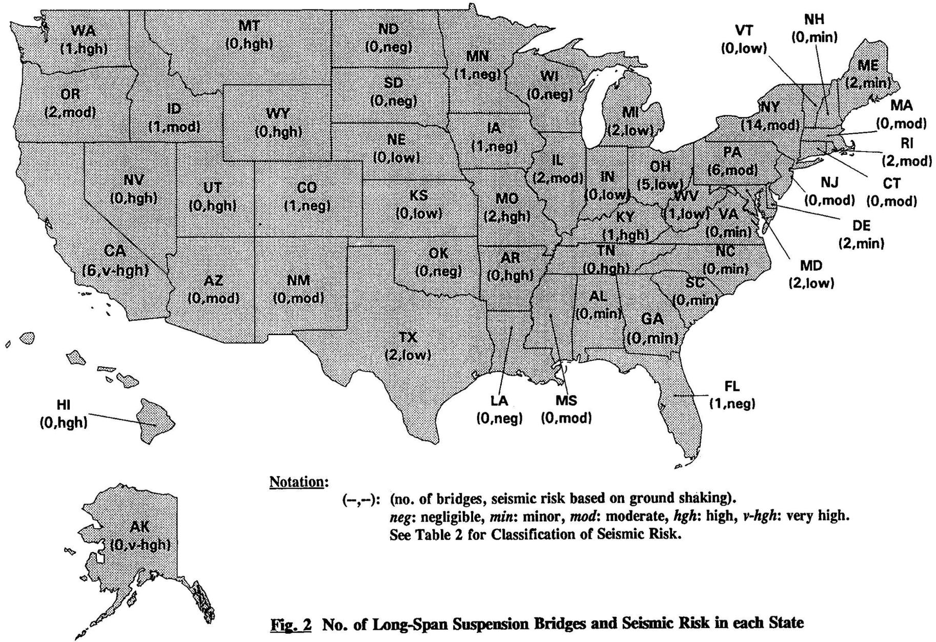
**Fig. 2** No. of Long-Span Suspension Bridges and Seismic Risk in each State
