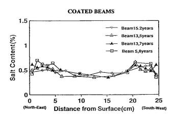
Fig. 3 Chloride distribution in beams with 0.5% salt
