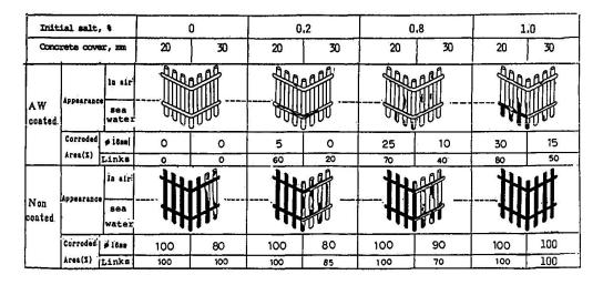
Fig. 1 Effect of AR coating on steel corrosion after 8 years' exposure
