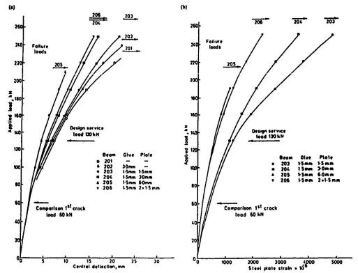
Fig. 4 Effect of bonded plates on mid-span deflection
