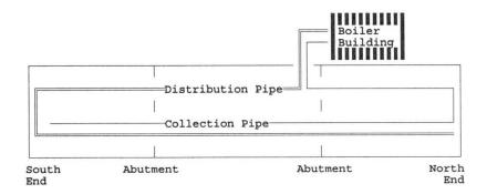
Fig. 2 Distribution/collection Network Schematic
