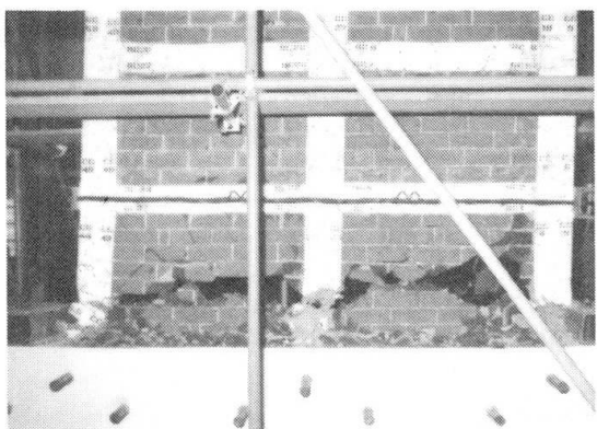
FIG.10. SPALLING OF BRICKS
