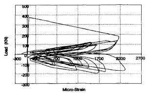
Fig. 5 Load-Rebar Micro Strain of PC-1
