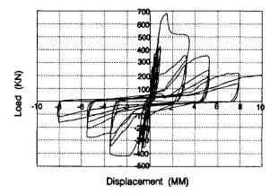
Fig. 6 Load-Interface Slip of PC-8
