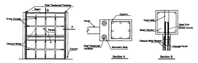
Fig.1 Precast Infill Wall System
