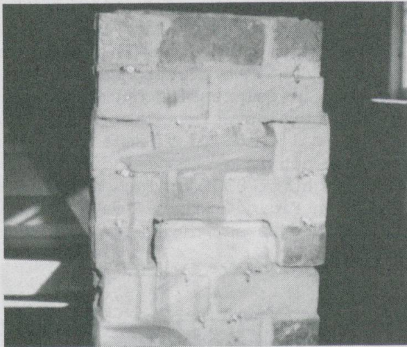
Fig. 6 Cracked wall with sheath
