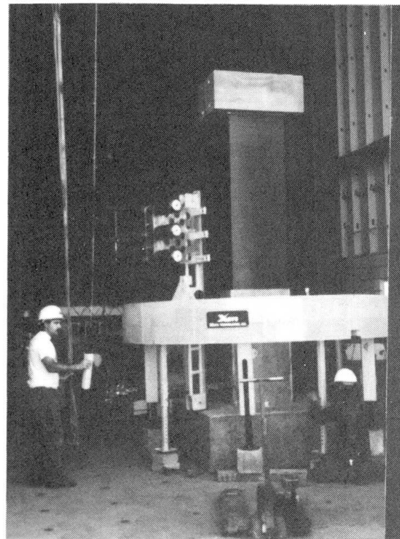
Fig. 1 Automated Carbon Jacket System
