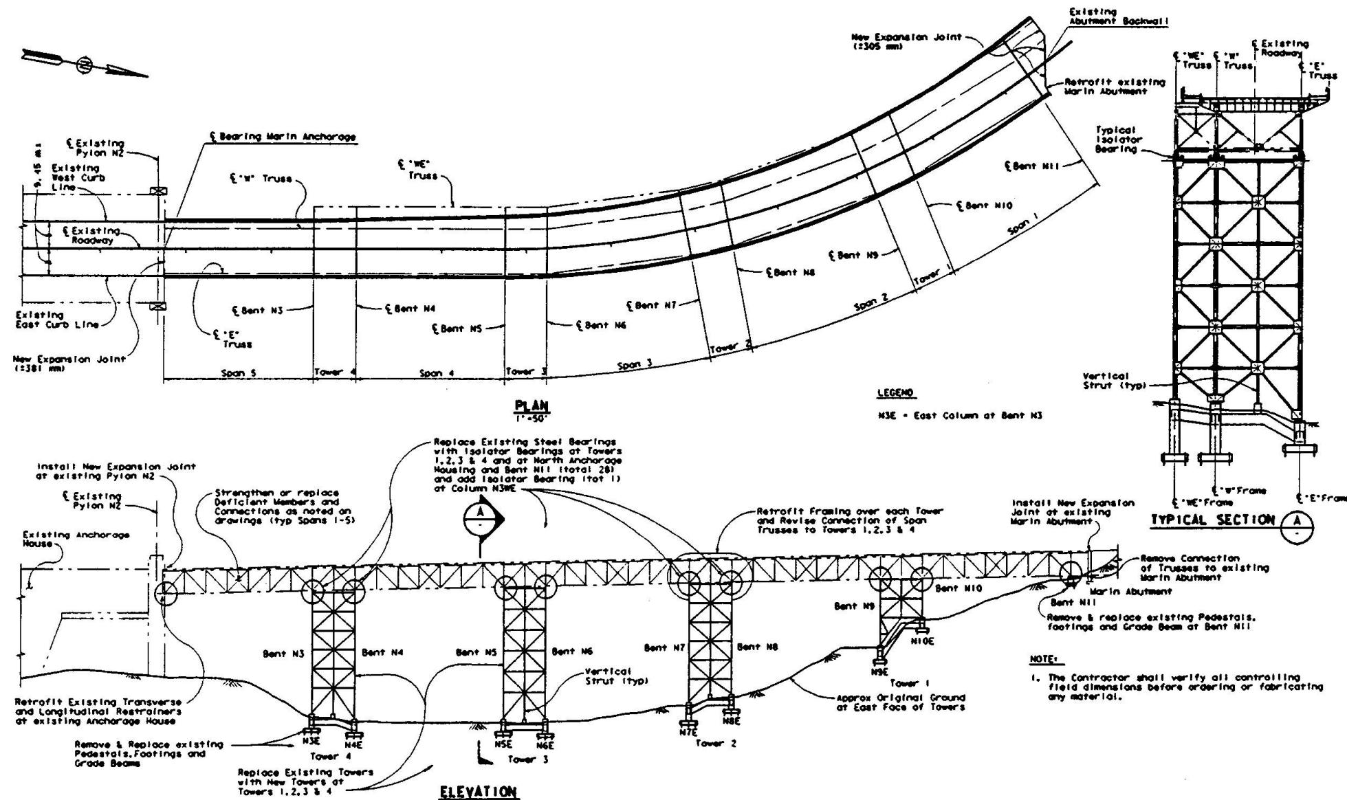
Figure 1 Seismic Retrofit of the North Approach Viaduct
