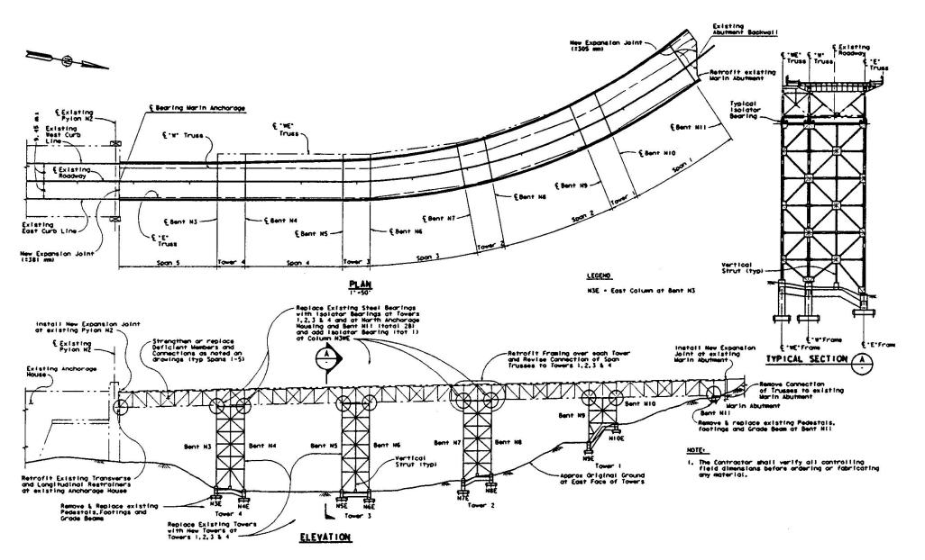
Figure 1 Seismic Retrofit of the North Approach Vioduct
