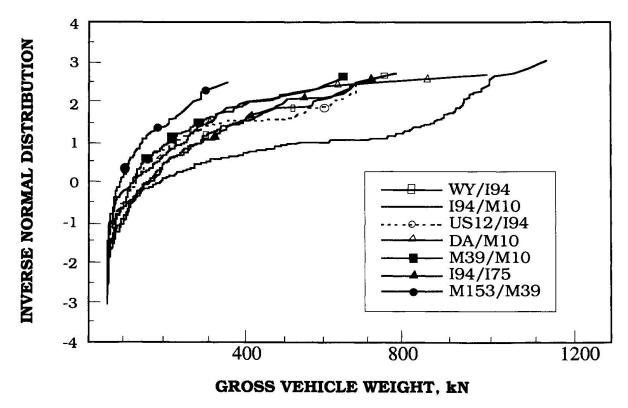
Fig. 1. Distribution Functions of Gross Vehicle Weight.
