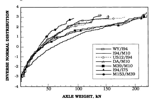
Fig. 2. Distribution Functions of Axle Weight.
