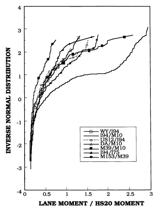
Fig. 3. Distribution Functions of Midspan Moments.
