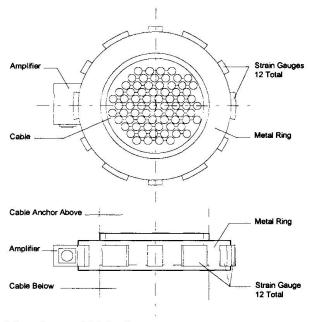
Fig. 6 Cable forces sensor
