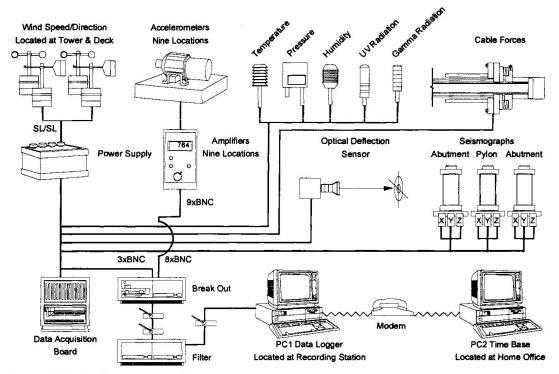
Fig. 5 Monitoring system diagram
