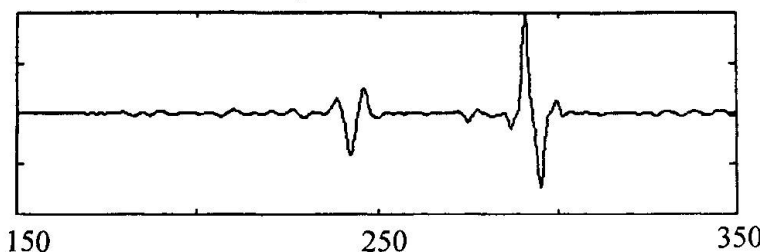
Fig. 9. Echo signal after Split Spectrum Processing versus time t [ \mu s].
