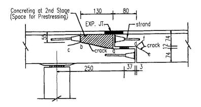
Figure 5. Cracks on Connection Joint
