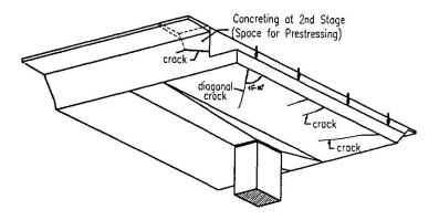
Figure 6. Cracks on Bottom of Connection Joint
