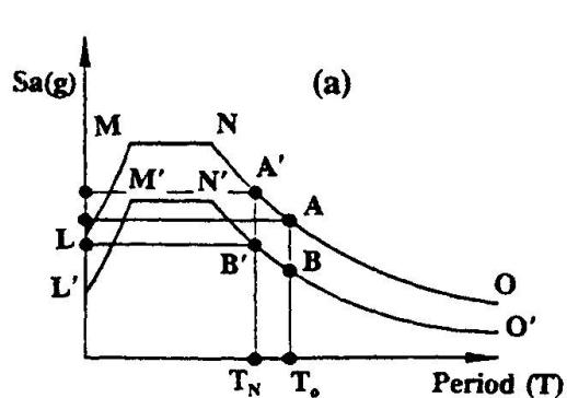
Fig. 1 (a) Schematic Spectrum for VE-System, and (b) Energy Idealization.
