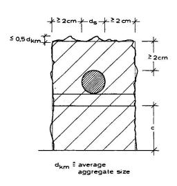
Fig. 5 Groove geometry
