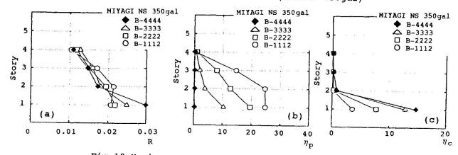
Fig.10 Maximum response of B-frame(MIYAGI 350gal)
