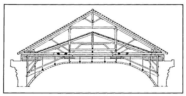
Fig. 3 Covering section after intervention: in evidence (down from above) upper trusses, lower trusses, steel prosthesis and the wooden vault now suspended to them.
