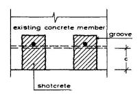
Fig.4 Additional reinforcement in grooves
