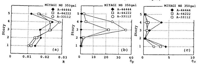
Fig. 12 Maximum response of A-frame(MIYAGI 350gal)
