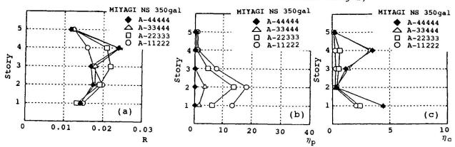
Fig.11 Maximum response of A-frame(MIYAGI 350gal)
