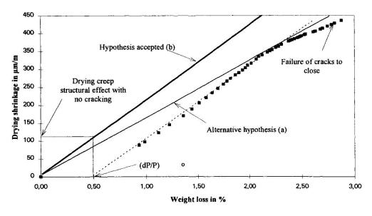
Fig. 2 Drying shrinkage versus weight loss.
