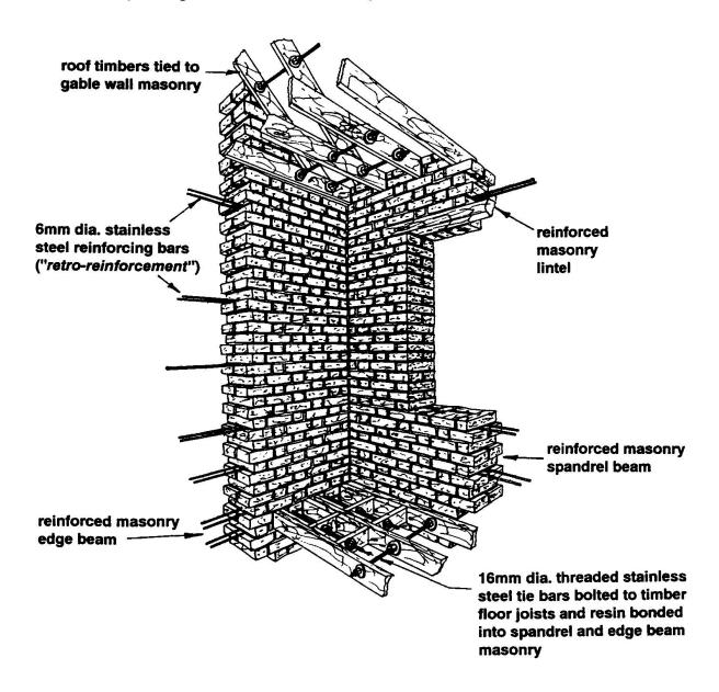
Fig. 1 Typical retro-reinforcement repairs to low-rise masonry construction
