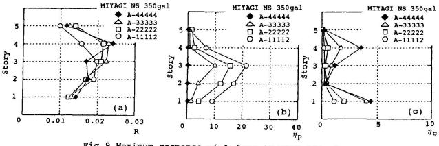
Fig.9 Maximum response of A-frame(MIYAGI 350gal)
