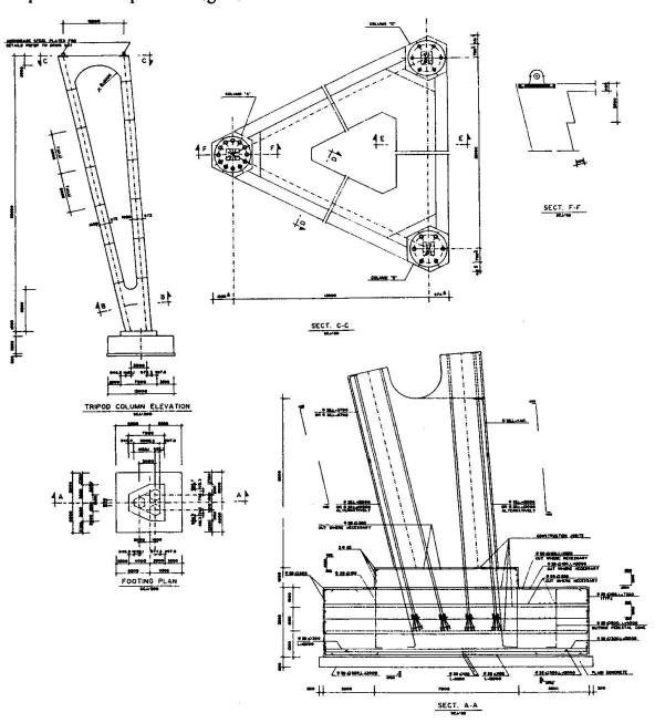
Fig. 2 Prestressed concrete column solution.
