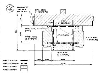
Figure 2 - SW1 Complex Retrofit Plan
