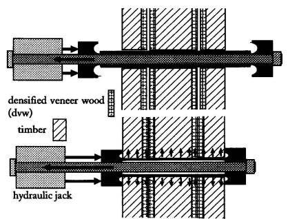
Figure 2: The principle of the prestressing procedure
