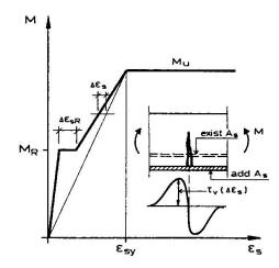
Fig.2 Changes in steel strains during cracking
