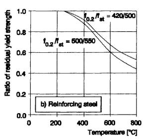
Fig. 1 Residual strengths of concrete and reinforcing steel as a function of temperature reached
