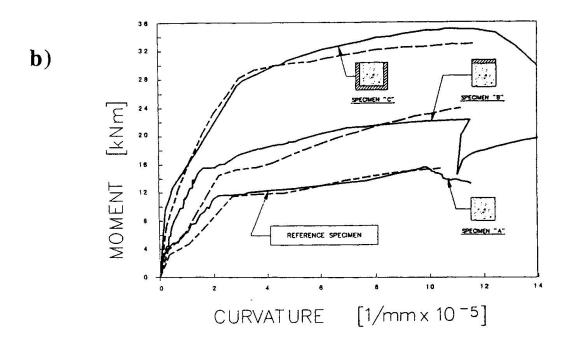
Figure 2: (a) Response of SIMCON in tension. (b) Experimentally (solid line) and analytically (dashed line) obtained moment - curvature behavior of reinforced concrete beams. Letters "A," "B," and "C" denote specimen types defined in Figure 1b.
