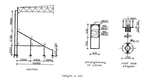
Fig. 2 Strengthening of reinforced concrete structures
