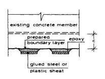
Fig.3 Additional reinforcement at the boundary layer
