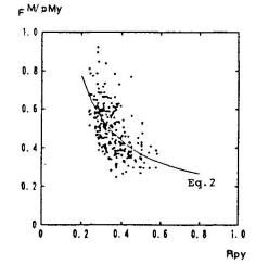
Fig.1 FM for practical sections (X-type with scallop)
