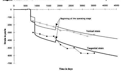
Fig. 5 Comparison between simulations and in situ measurements over a 10-year period.
