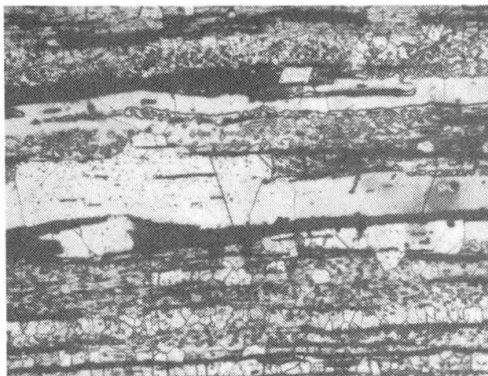
Fig. 2: Microstructure of wrought iron (L-S orientation, magn. 50x)
