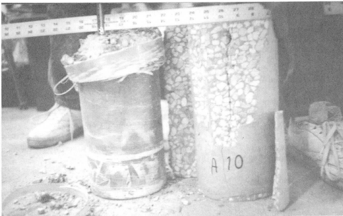
Fig.4 Control and Composite Specimens after Failure
