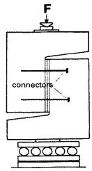
Fig. 5 Shear test (Walraven [4])
