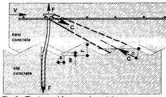
Fig. 3 The trussed framework model
