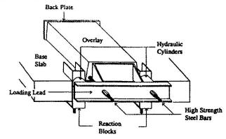
are of note: It is best for the trussed Fig. 4 Shear test (Choi [9])
