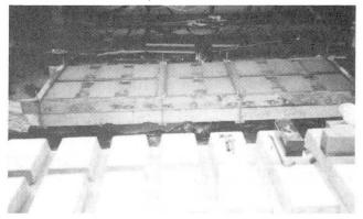
Fig. 8 In-situ shear tests of Hilti Jumbo Nails
