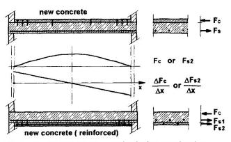
usually placed as cast- or pneu- <u>Fig. 1</u> Examples for the method of strengthening matically-placed concrete. It can work to augment either the flexural compression or tension zones, depending on reinforcement and placement (see Fig. 1).
