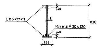
Fig.1 Dimensions of the built-up I-shaped stringers.
