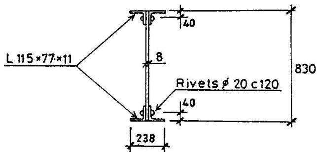
**Fig.1** Dimensions of the built-up I-shaped stringers.
