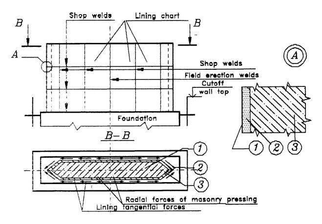
Basic circuit arrangement of steel lining piers Fig.1
