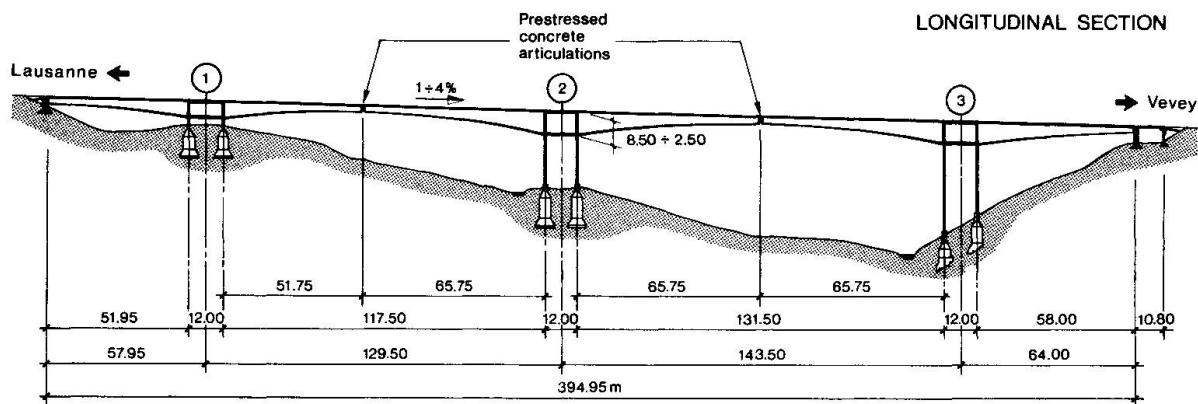
Figure 3: Longitudinal section of Lutrive South bridge
