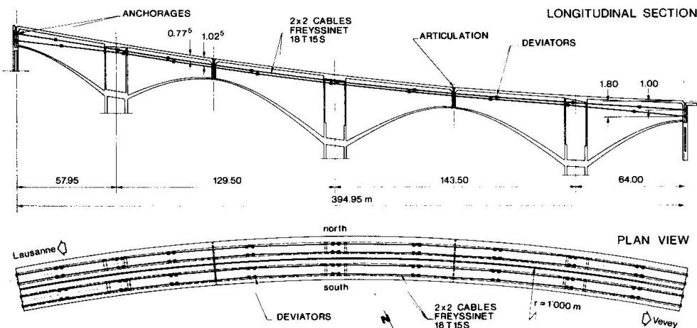
Figure 6: Scheme of the strengthening additional prestressing
