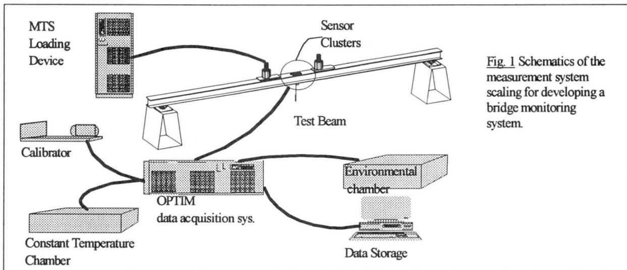
Fig. 1 Schematics of the measurement system scaling for developing a bridge monitoring system.
