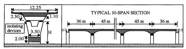
Fig. 1 - General lay-out of the "Coltano" bridge
