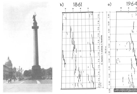
Fig. 2 Alexander's Column: a)- general view; b,c)- granite fust flaw fixing drawings
