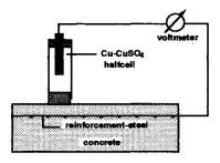
Fig. 1 Potential monitoring by means of Cu - CuSO<sub>4</sub> half-cell.
