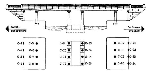
Fig. 3 Petrovsky Bridge in Schlisselburg: construction scheme
