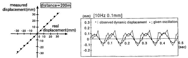
Fig.3 Linearity of the static displacement
