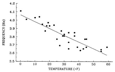
Figure 5 Frequency vs. Temperature for First Bending Mode
