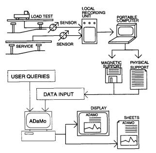
Fig.8 General scheme of the monitoring system
