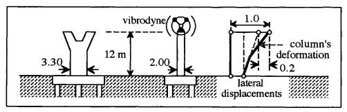
Fig. 2 - Dynamic test of a pier before the construction of the deck structure
