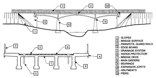
Fig. 1 The bridge components for which damage was monitored
