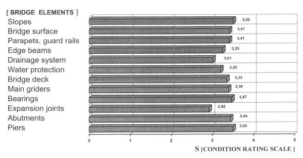
Fig. 3 Mean rates of the technical condition for the particular bridge components
