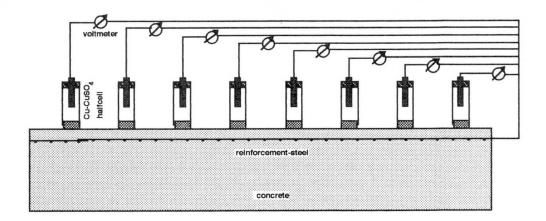
Fig.2 Monitoring system with 8 monitoring cells applied with a bridge construction
