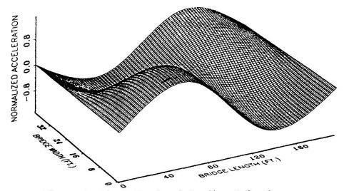
Figure 4 First Torsional Bending Mode Shape
