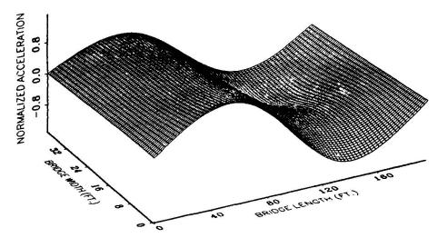
Figure 3 First Bending Mode Shape
