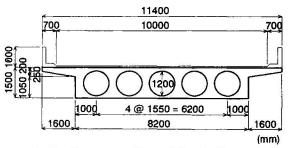
Fig.8 Cross section of the hollow girder
