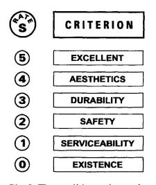
Fig. 2 The condition rating scale in Polish BMS
