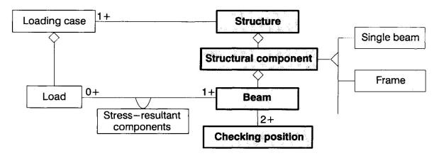
Fig. 4: Partial object model of the engineering application "Design and code verification"
