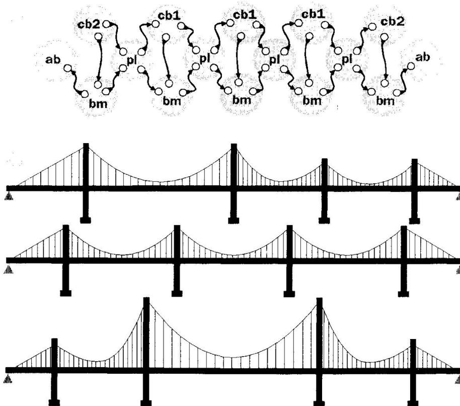
Fig. 3 A two stage description: a) the CP-graph representing topological features of potential bridges, b) three bridges specified by three different realization schemes for that CP-graph.
