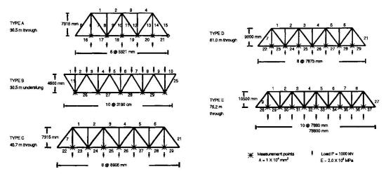
Figure 1: Configurations of steel railway bridges
