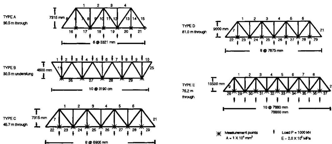
Figure 1 : Configurations of steel railway bridges
